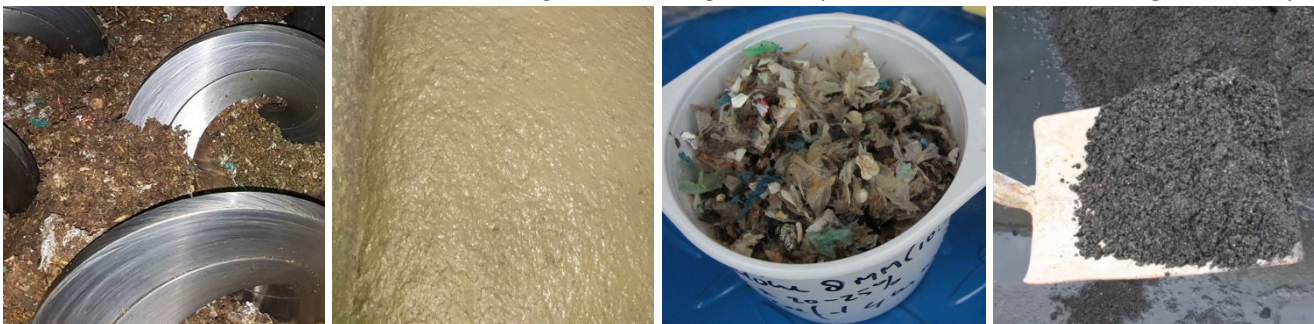
Figure 3: Input and Products from the Organics Polishing System (Left to Right) - Infeed from OREX™, Polished Wet Fraction, Light Rejects, Heavy Rejects
