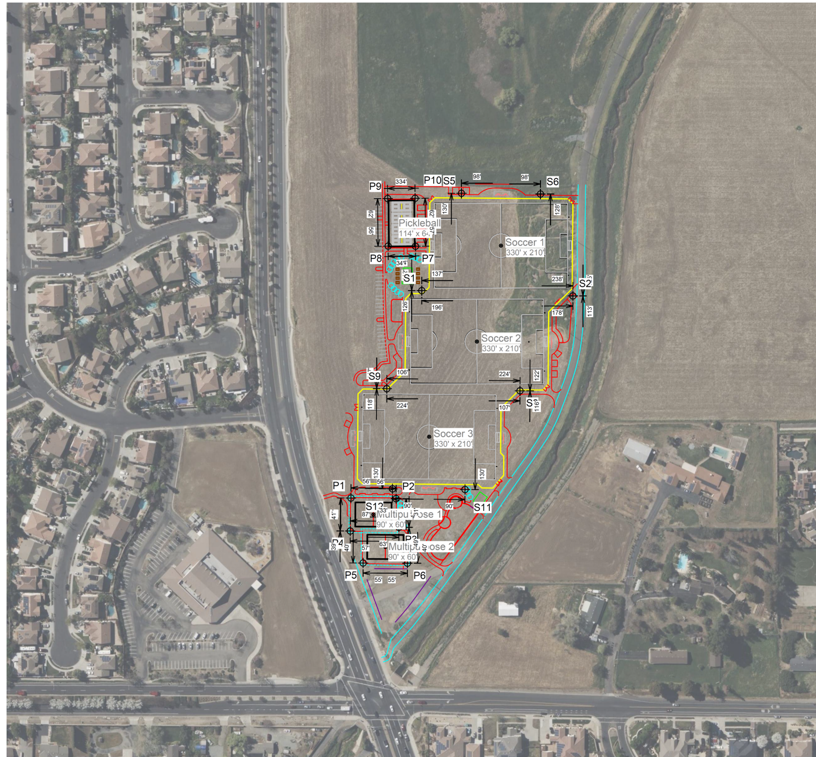
Figure 5 Illumination Equipment Layout
